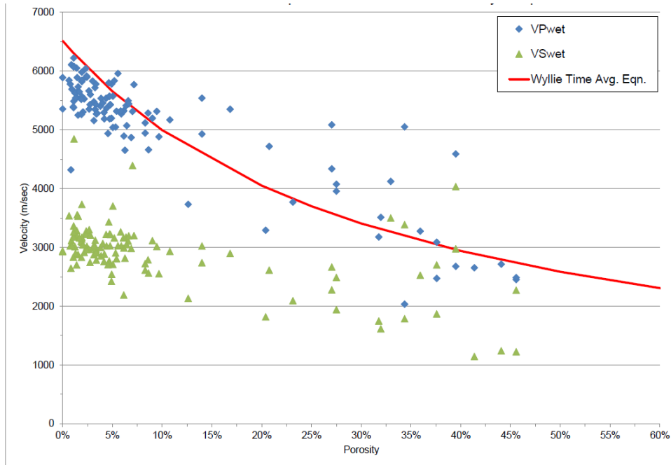
Figure V-8: The laboratory measured sonic velocity (acoustic response) data for samples from the Mid-Continent, Mississippian age samples shows a clear inverse relationship between the velocity and porosity for both compressional ( V_p ) and shear wave ( V_s ) responses. The relationship between the V_p response and the Wyllie time average equation plotted for values consistent with pure carbonate samples shows a distinct shift in the response for low porosity (<10%) samples. This is due to a difference in the mudrock mineral composition, the complicated micro- to nanoscale pore architecture, and the different type of grain coupling within a carbonate mudrock compared to conventional carbonates with predominantly macro- to mesopores.
