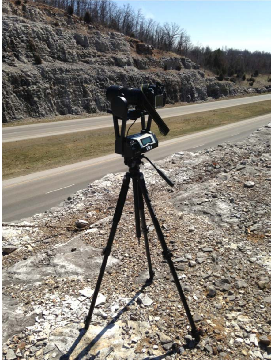
Figure 11: GigaPan® Epic Pro setup used for creation of high resolution giga-pixel images. The GigaPan® is an automated device that positions the camera at equally spaced user defined intervals while remotely capturing a picture at each interval. The output is a large number of overlapping images within a grid of rows and columns. GigaPan Stitch™ software is then used to piece together the photographs. The program first aligns the pixels of each image to identify how they overlap. It then stretches and rotates each image to make them align. The program then blends the images into one seamless high resolution panorama ( www.gigapan.com ).
