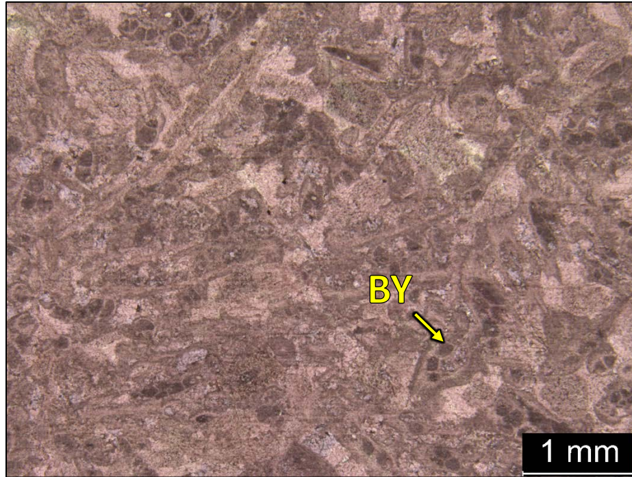
3 TF – 5347.5' : Bryozoan grain rich packstone to grainstone. Sample is alizarin red stained (half slide) and blue epoxy impregnated. Porosity (NCS): 0.8%. Permeability (Klinkenberg): 0.0001 mD. Visual estimation: 2% clays, 98% carbonates. Sample contains bivalves (20%), brachiopods (2%), bryozoans (20%), crinoid fragments (15%) and undifferentiated skeletal debris. Slight intraparticle porosity observed.
