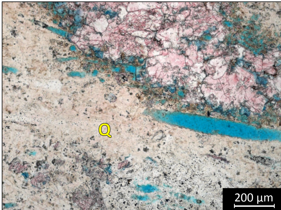
1 BN – 5255.90' : Bioturbated wackestone to packstone. Sample is alizarin red stained and blue epoxy impregnated. Porosity (NCS): 12.7%. Permeability (Klinkenberg): 0.323 mD. XRD: 0.5% clay (illite+mica), 56.1% carbonate (calcite), and 43.4% other minerals (43.2% quartz and trace amounts of pyrite and halite). Sample contains crinoid fragments
