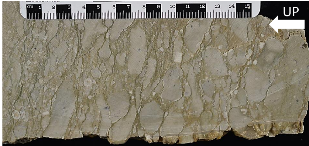
Figure 36: Sample of the debris flow bed within the Compton Formation. Mud clasts ranging in grain size from very coarse sand to very coarse pebbles (2 mm – 2.5 in) are set within a crinoidal-bryozoan micrite matrix very similar to the composition of the Compton Formation. Note the scale is in centimeters and the up direction is to the left.
