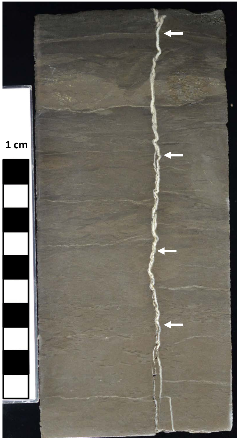
Core photo of ptygmatic fracturing (arrows) in the Elinore core in Facies 3 (bioturbated wackestone-packstone) at a depth of 4458.4'. The fracture height is approximately 450 millimeters and the aperture ranges from 0.1-2 millimeters. The fracture is mineralized
