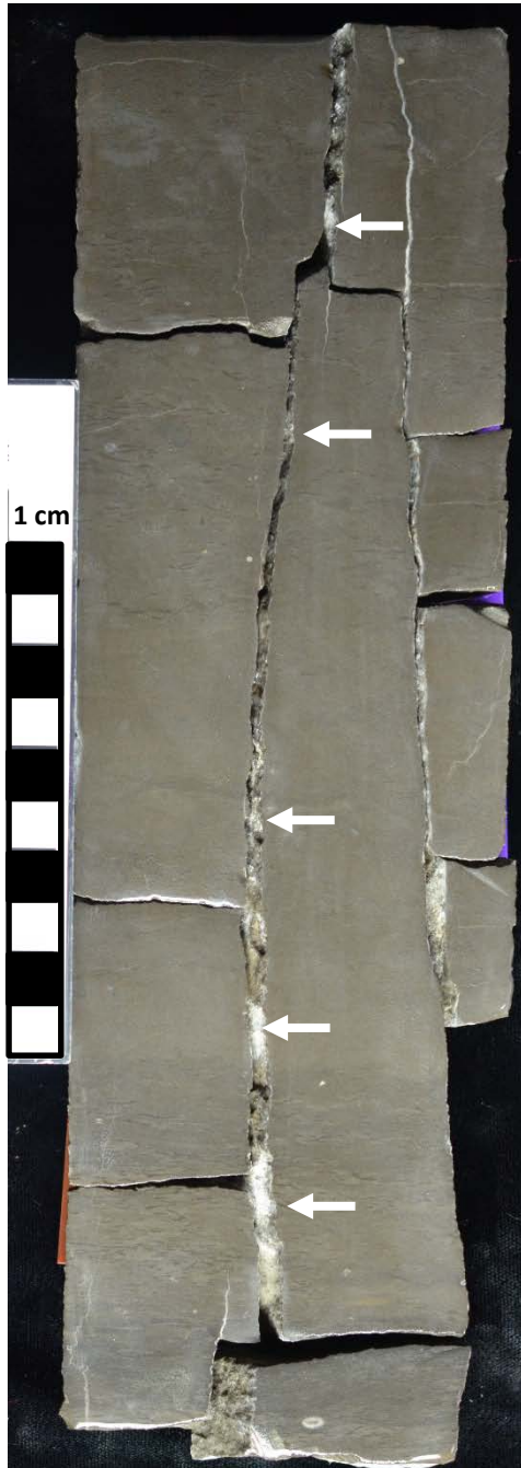
Core photo of vertical extensional fracturing (arrows) in the Elinore core in Facies 3 (bioturbated wackestone-packstone) at a depth of 4459.0'. The fracture height is approximately 335 millimeters and the aperture was not measured due to the fracture
