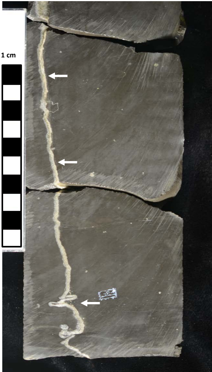
Core photo of ptigmatic fracturing (arrows) in the Orion Blackbird core in Facies 2 (burrowed mudstone-wackestone) at a depth of 3406.2'. The fracture height is approximately 189 millimeters and the aperture ranges from 0.5-4 millimeters. The fracture is mineralized with calcite and heavier folding occurs near the bottom of the photo.
