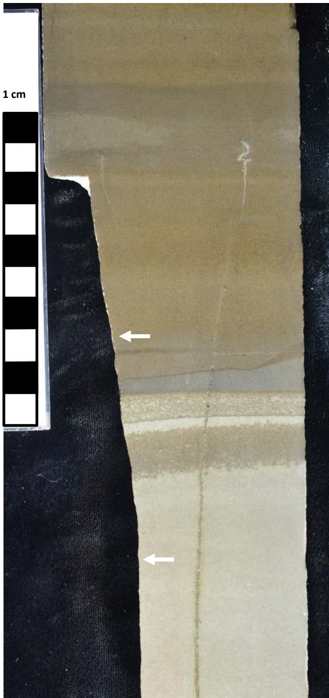
Core photo of vertical extensional fracturing (arrows) in the Elinore core in Facies 4 (crinoidal packstone-grainstone) at a depth of 4411.5'. The fracture height is approximately 291 millimeters and the aperture was not measured due to the fracture
