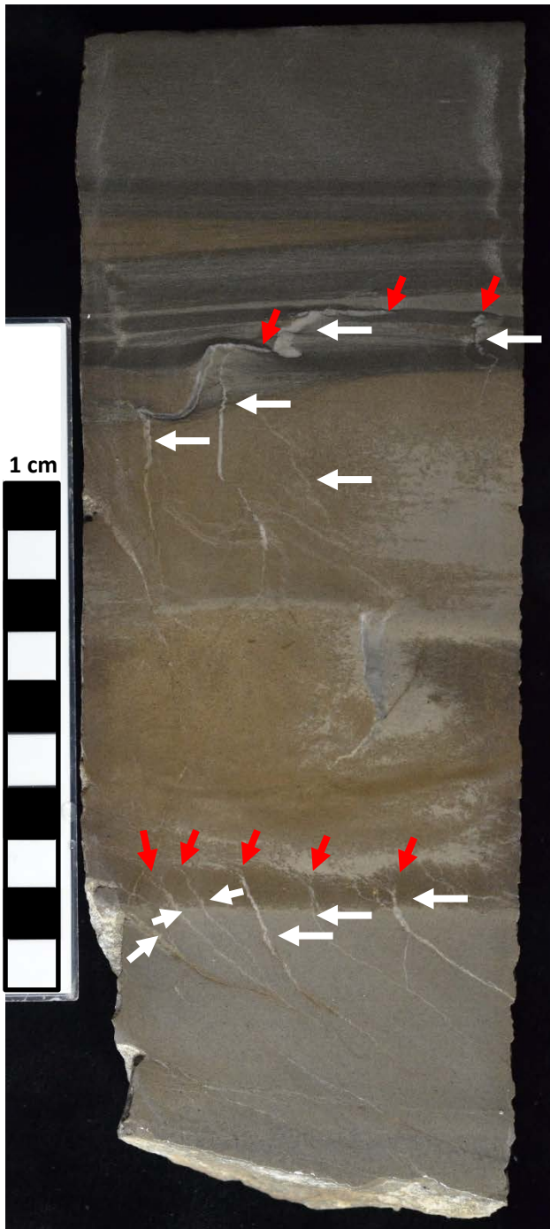
Core photo of ptymatic fracturing in the Elinore core in Facies 4 (crinoidal packstone-grainstone) at a depth of 4395.3'. The ptymatic fractures are indicated by the white arrows. The fracture heights range from 20-35 millimeters and the apertures range from 0.1-1.5 millimeters. The fractures are mineralized with calcite and the red arrows
